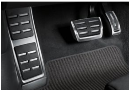
Foot rest and pedal caps in stainless steel and the footrest made of brushed stainless steel.
